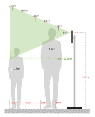
Recommended Installation Height: 150cm Temperature Measurement Distance: 30cm to 120cm
