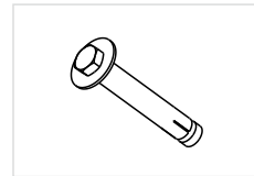
Internal Expansion Anchor 100x16xM12mm (Qty 11)
